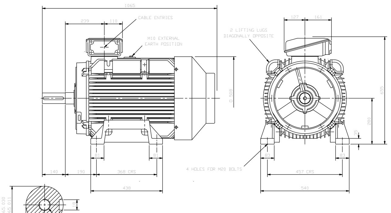
TERMINAL BOX CAN BE SIDE MOUNTED (LEFT OR RIGHT) BY REFITTING FEET 90° IN APPROPRIATE DIRECTION. CABLE ENTRY CAN BE SUPPLIED IN ANY ONE OF FOUR POSITIONS AT 90° INTERVALS.
